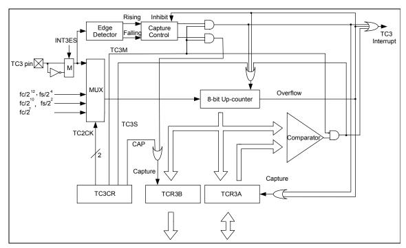
Fig. 5-22 Configuration of Timer/Counter3
